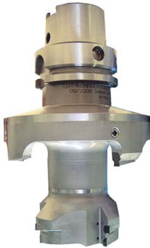
Figure 4: PCD-equipped bell tool for drilling/reaming and countersinking (source: LMT Group)
