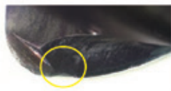
Defect due to high load
