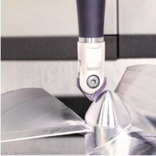
Fig. 3 – One insert barrel-shape cutters demonstrate high performance parameters when machining complex surfaces of vital components.
