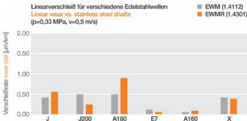
The wear test in the in-house igus test laboratory demonstrates that the liner made of iglidur A160 is the optimum sliding partner for stainless steel shafts.
