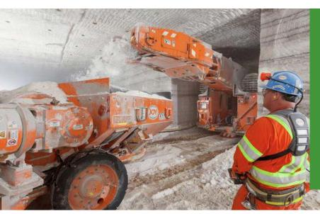
Highfield Resources' Muga project in northern Spain is expected to produce 1Mt of MOP per annum, following two phases of development. The company will use traditional underground room and pillar mining, with declines providing access to shallow mineralisation. Processing will be via conventional flotation and crystallisation.
