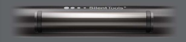
Inside the tool is a pre-tuned damping system that consists of a heavy mass, supported by rubber spring elements. If vibration arise, the kinetic energy will be absorbed by the damping system. This leads to minimized vibration and greatly improved productivity.
