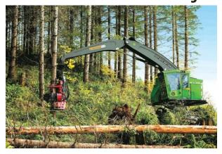
o help loggers maximise timber quality, John Deere has upgraded its harvester stick boom attachment across all 800MH- and 900MH-Series tracked harvesters.
