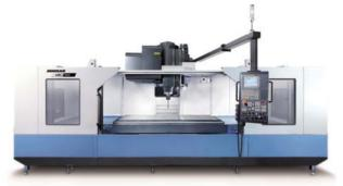
VM series VM 750 (L) / 960 (L) / 1260 Large, high-speed, high-precision machining center
