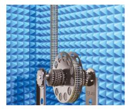
Tests conducted in the 2,750 square metre test lab demonstrated the low noise emissions of the e-spool. Thus, the cable reel without slip ring qualified for low operation noise in the stage sector. (Source: iqus GmbH)
