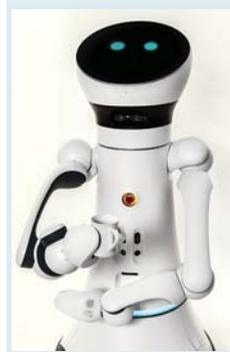
The standardised Schunk Powerball Lightweight Arm combined with the one-finger hand allows various gripper operations. Source: Fraunhofer IPA, Photo: Rainer Bez
