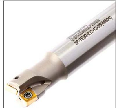
are also available overcut diameter sizes 13mm, 17mm and 21mm to facilitate deep cavity or shoulder machining. 2PKT 05 inserts are available in 2 geometries, “M” for general purpose machining applications and “ML” for low power machining in unstable setups and long overhangs.
