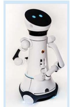
The modular design of Care-O-bot 4 allows the set-up of an individual robot platform for various applications, decisively reducing the costs for developing new service robotics solutions. Source: Fraunhofer IPA, Photo: Rainer Bez
