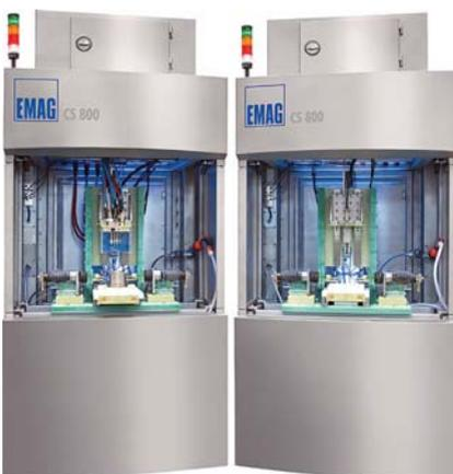
View of a complete ECM cell for the drilling process.
