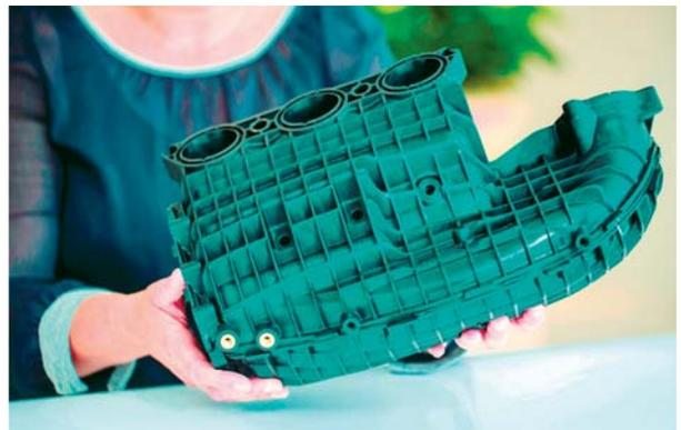
Stanyl Diablo PA46 delivers performance on the world's first high-heat plastic air intake manifold with integrated charge air cooler.
