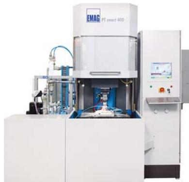
**The ECM laboratory machine PTsmart can be found at the laboratory facility in Gaildorf. On it, detailed preliminary studies establish the feasibility of the process, whilst other EMAG staff determine the cost-benefit ratio of ECM in comparison to other methods.**
