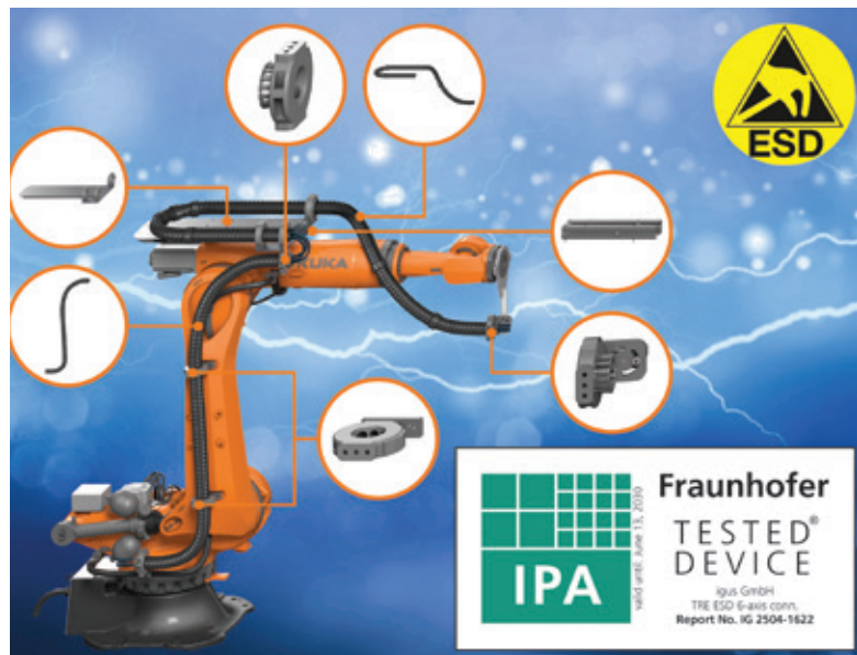
With the triflex TRE ESD, igus is launching the world's first ready-to-connect dress pack that is ESD-capable as a complete system. (Source: igus GmbH)
