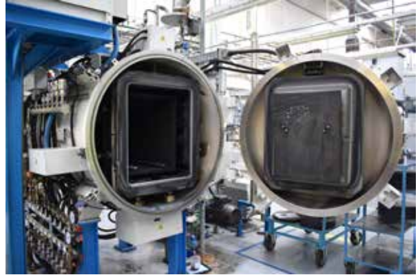
The sintering furnace at Dormer Pramet's indexable production unit.
