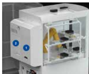
Robot loader with the externally installed tool cleaning (1) and laser marking modules (2)
