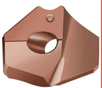
The new Color Select P6005-WKK45C indexable insert for Xtra-tec<sup>®</sup> point drilling and boring tools has been optimised for use with cast iron workpieces. Walter manufactures this insert with a diameter of 12 to 29,77 mm. The colour of its coating indicates which ISO material group it should be used with. *Image: Walter AG*
