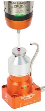
Global engineering technologies company Renishaw has launched the Primo<sup>™</sup> LTS (length tool setter) at CIMT, Beijing, China. The Primo LTS is a single-axis tool setter which allows users to set tool length, check for breakage, and compensate for thermal growth on a CNC machining centre.
