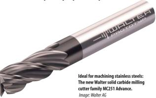
provide a high level of machining reliability. And because the coating is made from a combination of titanium aluminium nitrate (TiAlN) and aluminium titanium (AlTi), not only is the tool's service life extended significantly, but it also exhibits particularly good anti adhesion properties, which means that the formation of build-up on the cutting edge is not significant.
