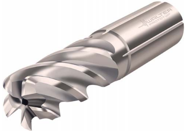
The Walter Prototyp Ti40 is the titanium specialist among solid carbide end milling cutters. Its differential tooth pitch and the special design of the edge counter vibration. The tool is also suitable for intelligent strategies such as high dynamic cutting. Image: Walter AG
