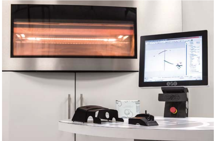
Mercedes-Benz Trucks already successfully produces 30 spare parts with the latest 3D SLS printing processes.
