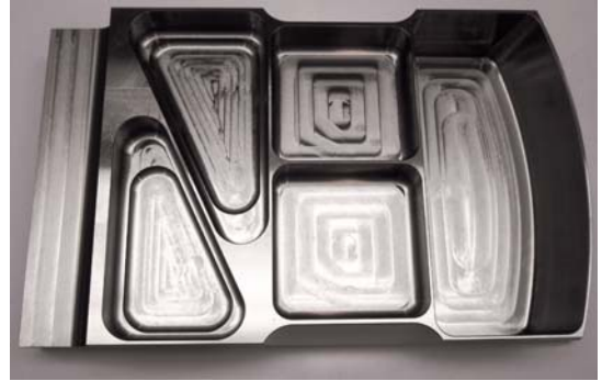
Using a generic component made from Ti6Al4V, the aerospace experts at Walter AG demonstrated typical processes for structural components. Image: Walter AG
