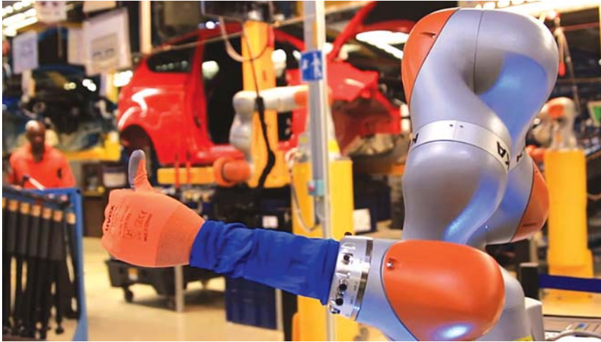
New collaborative robots, also known as co-bots, are first being used to help workers fit shock absorbers to Fiesta cars, a task that requires pinpoint accuracy, strength, and a high level of dexterity. Employees work hand-in-hand with the robots to ensure a perfect fit every time. Courtesy: Ford
