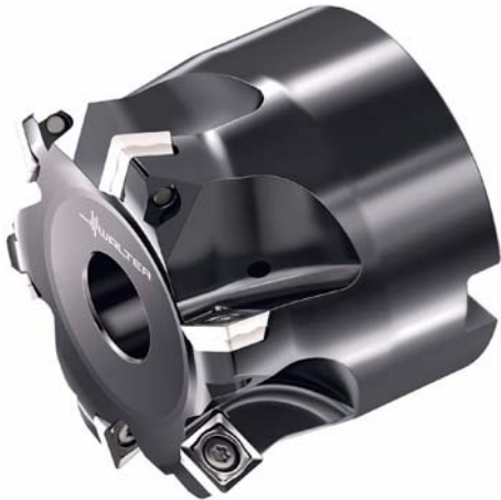
The M4002 is a high-feed milling cutter suitable for facing, interpolation and part plunging. The lead angle on the universal inserts is 15°. Equipped with the WSM45X cutting tool material, this tool is the ideal solution for pocket machining on components made of titanium. Image: Walter AG
