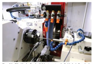
View of the S33 with wheelhead, which has two external cylindrical grinding wheels here. An internal grinding spindle could also be integrated as a modular unit.
