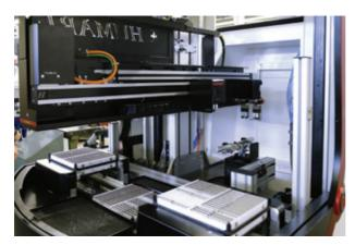
For machining around the clock: The blanks and finish-machined recirculating ball screws are 'handled' by 3-axis linear robots.
