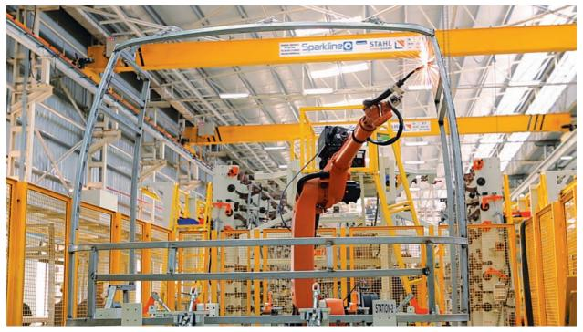
The plant also has robotic welding facilities for main body and under body welding
