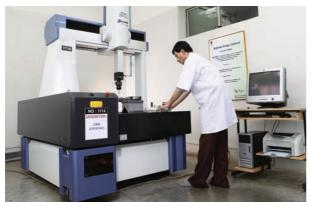
Co-ordinate Measuring Machine for checking critical machining dimenions.
