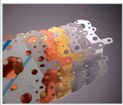
The TruLaser 1030 fibre cuts not only aluminium, stainless steel and mild steel, but copper and brass, as well. Trumpf India.
