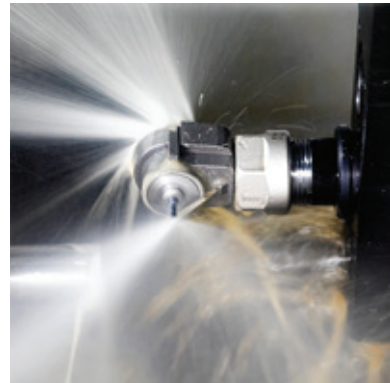
Figure 5: Compact MICRO 90 coolant-driven spindle is an effective tool to boost the rotational velocity of miniature cutting tools.
