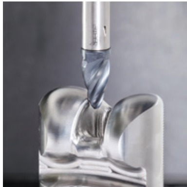
Figure 4: Applying small-in-diameter barrel-shaped endmills significantly reduces cycle time when machining the components of a knee prosthesis.
