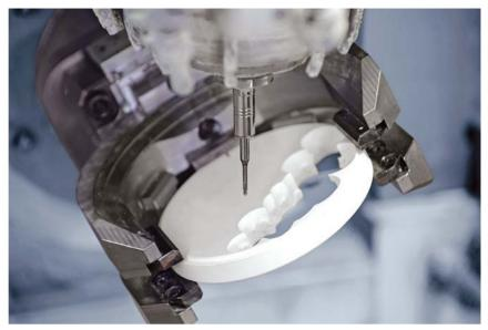
In the field of dental technology the TRIBOS polygonal technology is used for milling zircon at maximum precision.
