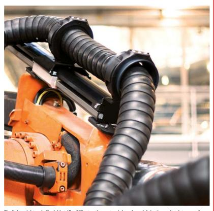
The lightweight and affordable triflex RSE retraction system is based on a lubrication and maintenance free drylin linear guide from igus. A moving carriage transports the chain, elastic cords keep it under tension and retract it automatically. (Source: igus GmbH)
