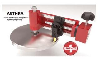
Ø 1" to Ø 6". The main components of this facer, like arm, housing, is cast from Aluminium to make it light. Sliding surface is made of LM guides and blocks to provide utmost frictionless smooth movement, keeping in mind the operator's fatigue. The tool is moved over the LM guides through a leadscrewbox nut arrangement,
