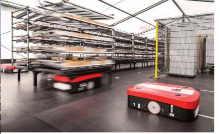
Driverless transport systems supply parts autonomously
