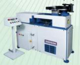
HYDRAULIC PIPE & TUBE BENDING M/c. Capacity: Upto 100mm Thickness Upto 6 mm (M.S.)
