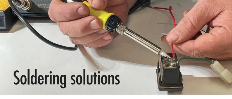
s outlined in last month's *Workshop* article, soldering really is the best way to reliably join electrical connections. It forms a very low-resistance electrical connection, and if done properly, moisture cannot get in between contact surfaces causing corrosion and increased resistance to current flow.
