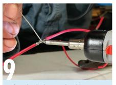
With good quality batteries, the soldering iron surprisingly performs quite well, and is perfectly suitable for soldering smaller automotive wires or even repairing kid's toys. Having no power cord, it is quite convenient to use. Tradeflame also makes a similar unit which is rechargeable via USB connection, and costs \$90.
