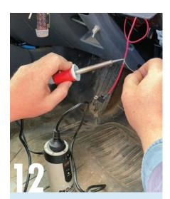
You may already have all the equipment on hand for soldering away from the workshop. A perfectly workable setup is the use a 12V to 240V inverter, and a low-cost soldering iron as shown. An extension cord can be used if you need to solder away from the power source. It may not be as fast as the Milwaukee cordless soldering iron but it will get the job done.
