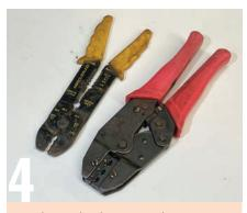
A quality set of ratchet crimping pliers is a must (right) and is sized for the correct amount of pressure for red, blue and yellow crimp connectors. Avoid cheap crimping pliers (left) as they do a second-rate job. The wire stripping section in between the handles actually works better than the crimping jaws.
