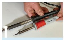
Most of us will have a couple of low-cost basic 240V soldering irons in the workshop. They will carry a current rating such as 25, 40 or 50W which is a direct measure of the amount of heat it can output. Larger capacity soldering irons will usually have a larger tip, or will be provided with an interchangeable chisel tip or point tip. Most will only have a fixed output so a larger unit may cause problems with smaller wires such as melting the insulation.
