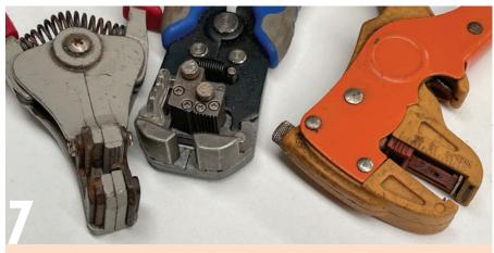
There are plenty of different style wire strippers available, and selection is largely based on user preference. While stripping pliers are not essential, they save time when stripping multiple wires. Select a pair with adjustable pressure and strip length.
