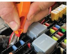
While you can easily check continuity with a multimeter, the fuse tester can be simply pressed against the back side of a blade fuse while it is in place (left). If you need to remove the fuse, the jaws on the other end make it easier to grip (right).
