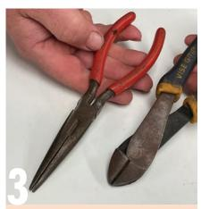
While on the subject of pliers, any electrical toolkit will benefit from a set of needle nose and side cutter pliers. Needle nose pliers are ideal for any fiddly, delicate work, and for any the side cutters are a little easier to use for cutting cable.
