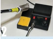
A better option for the workshop is a soldering station with adjustable output. The tip temperature can be tailored for the size of the job or the melting point of the solder used. This unit has a maximum output of 48W and cost about \$110, although you can spend several hundred dollars for higher output soldering stations with more advanced features and digital displays.
