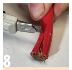
Keep a sharp knife or box cutter in your kit. Apart from being useful when peeling insulation off larger cables it will come in handy for all sorts of jobs.
