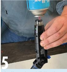
The soldering torch is simply filled from a butane can by pressing against the base with the unit held upside down. A refill can costs about \$10 and will provide several refills.
