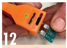
While there are plenty of different testers which can be included in your electrical toolkit, we found this Narva fuse tester and remover particularly handy. It has a set of adjustable pins which can be used to check the continuity of different size blade fuses.
