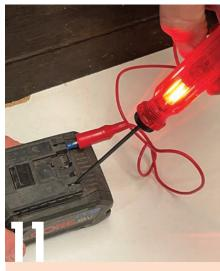
If multimeters aren't your thing, a test lamp will help with some fault-finding tasks. They are also quick and easy to use as one lead can be clipped on to a terminal (or earthed vehicle chassis) and the probe quickly touched onto a terminal, or even carefully used to pierce the insulation of a cable to contact the wire underneath. The unit pictured handles voltages from 6 to 36V and costs around \$20.
