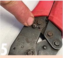
With use, the ratchet crimping pliers may require adjustment to increase the jaw pressure and make sure the jaws close fully when crimping. Remove the small screw pictured and advance the graduated adjusting wheel a notch or two as needed.
