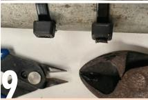
A pair of cable tie or flush-cutting pliers is a pretty handy tool to throw in. Cable ties are commonly used when securing electrical cables, but standard side cutters or other pliers will leave a sharp nib protruding when trimming the tie which can cause injury. The cable tie pliers leave the trimmed tail flush as shown on the left.
