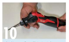
The ultimate cordless soldering iron is the Milwaukee 12V unit, which costs about \$169 for the skin (without battery). If you have any other Milwaukee 12V cordless gear, it would be a great addition, otherwise it will cost around \$300 in a kit with a charger and a single 2Ah battery. The unit has an impressive output of 90W and reaches operating temperature in 18 seconds, with a maximum temperature of 400 degrees Celsius.
