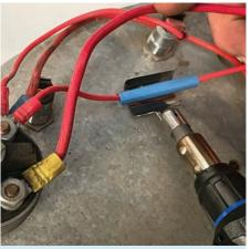
A benefit of the gas-powered soldering iron is that it can also be used as a heat source for heat shrink insulation. Simply remove the soldering tip while the unit is cool (left). This kit is supplied with a slip-on heat shield which can be used to protect other wires in close proximity from damage (right).
