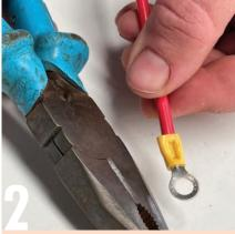
You can also use the crimping jaws in between the handles to compress crimp connectors, although it won't do as good a job as a dedicated set of crimping pliers. While it is irrelevant for 12V work, the handles are insulated to 1000V. This 216mm Channellock brand costs around \$65.
