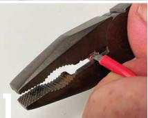
The cornerstone of any electrical toolkit is a pair of quality linesman's pliers. While they resemble standard pliers, there are a few key differences. The cutting jaws are of a 'knife and anvil' design, where one edge is blunt and the other sharp, which helps when stripping wire to avoid cutting through both the insulation and wire underneath. The gripping jaws are a crosshatch pattern which helps for gripping and twisting wire.
