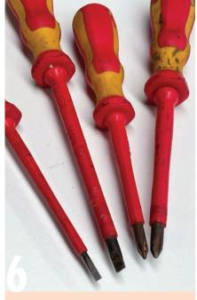
A set of electrician's screwdrivers is essential in any electrical kit. While the 1000V insulated shank is designed more for commercial electrical work, it can prevent accidental shorting when working on 12 and 24V electrical systems. While any appropriate sized screwdrivers can be used, dedicated electrical screwdrivers tend to have tips sized to common electrical terminal screws. A set of watchmaker's screwdrivers is also handy.
