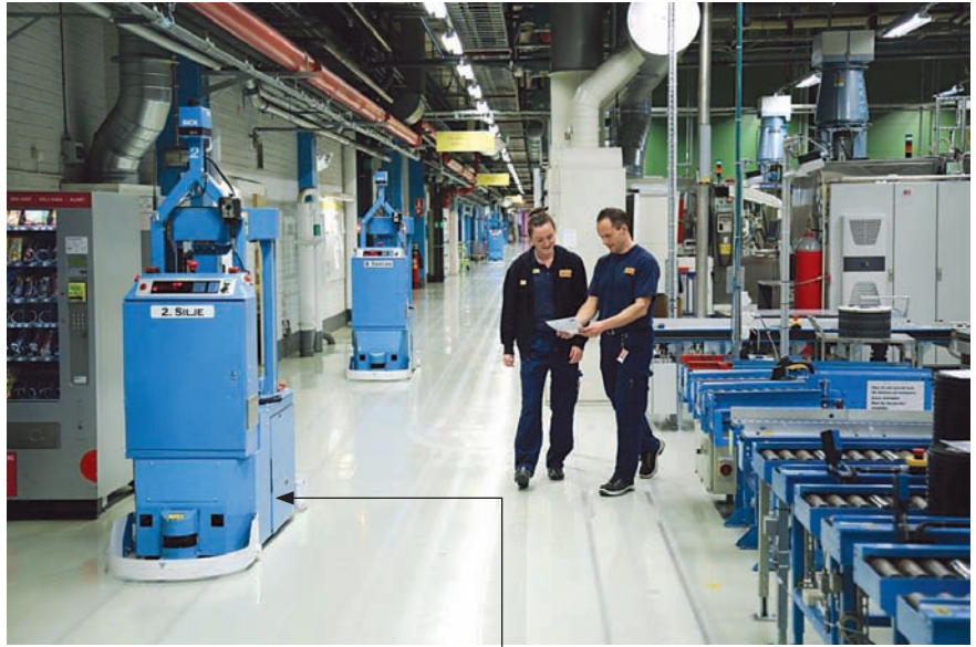
Inside Sandvik's Gimo plant where human beings and robots - blue coloured automated guided vehicles (AGVs) work together.
