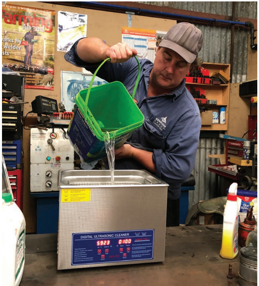
Ultrasound appointment: It sounds a bit like black magic, but ultrasonic cleaning has been in use for decades. The technology is now cheap enough to add to the farm workshop. Photos: Ben White and Josh Giumelli
