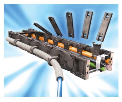
Neither screws nor tools are required for their attachment to the e-chain and the assembly of the corrugated tubes. Both assembly and disassembly are therefore very fast and easy. The e-chain and corrugated tube are joined together in the E4.1 TUBs, so that the whole system works very harmoniously offering a long service life.
