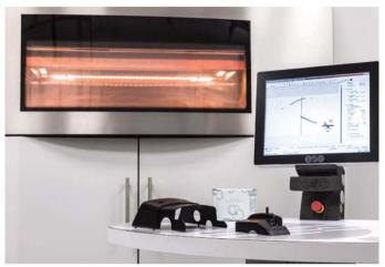
Mercedes-Benz Trucks already successfully produces 30 spare parts with the latest 3D SLS printing processes.
