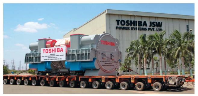
Toshiba JSW's first 'Made in India' 800MW Steam Turbine Generator for Unit 2 of NTPC's Kudgi Thermal Power Station
