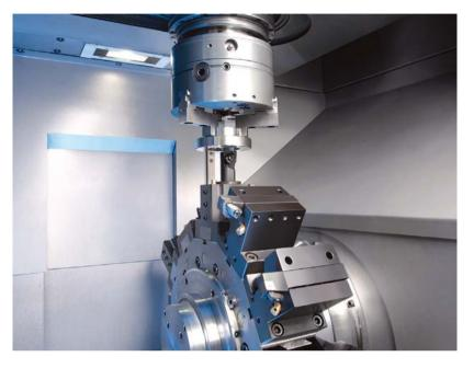
The working spindle is the heart of the pick-up automation system which is an essential part of every modular machine. It includes a parts storage unit in every machine, from which the pick-up spindle loads and unloads itself independently. This lowers non-productive time to an absolute minimum as there are only a few seconds between the machining processes.
