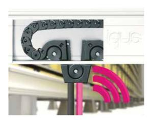
INTEGRATED "SIDE WINGS" HOLD THE CHAIN FIRMLY IN THE STRETCHED CONDITION AT ALL TIMES IN A SPECIAL GROOVE IN THE UPPER AND LOWER PART OF THE CHANNEL. TOGETHER WITH PLASTIC SPRINGS ON THE CROSSBARS OF THE E-CHAIN, THEY PROVIDE A SOFT AND QUIET ROLLING. THIS MEANS THE FRICTION, WEAR, ENERGY CONSUMPTION AND NOISE DEVELOPMENT ARE REDUCED SIGNIFICANTLY.
