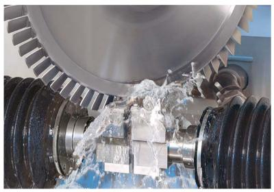
Machining area of an EMAG PO 900 BF for blisk machining using PECM (precise electro-chemical machining) technology
