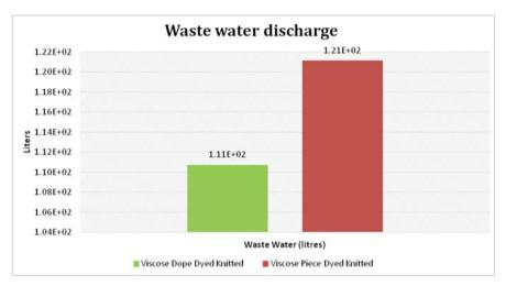
"In contrast to the traditional dyeing processes, Spunshades are manufactured with a technique that places colour pigments in the fibre itself when it is being made/spun – Spundyed. This eliminates the need for conventional piece dyeing and saves about 30 litres of water per meter of fabric processed."
