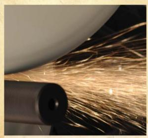
Uncontrolled heat build up can lead to discoloured and damaged components
