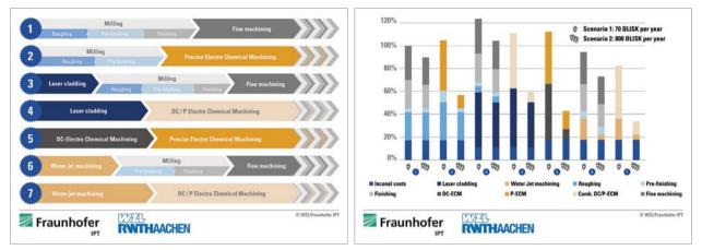
Seven different machining combinations were used in the study conducted by Fraunhofer IPT and WZL from RWTH Aachen. Complete mechanical machining (number 1) was used as the benchmark. The costs for an assumed volume of 70 BLISKs per year were 100 percent, failing to around 90 percent for 800 units (far left). In machining combination number 2 (rough milling and PECM), the costs falls to less than 60 percent. Source: Fraunhofer IPT/WZL
