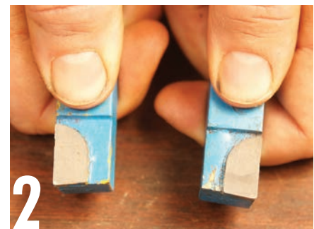
2 The tool can travel either left to right, or right to left and there are separate left or right-handed cutting tools to suit. Most turning is performed from right to left as this is the default travel direction on auto-feed systems.
