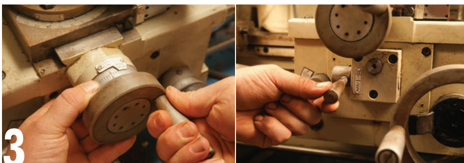
3 To turn down a shaft, set the spindle in motion and advance the tool until the tip just contacts the work. Set the micrometer sleeve on the cross slide handwheel to zero (or zero the digital readout unit). Advance the tool into the work the desired depth and engage the auto feed (right). Note that one complete turn of the handwheel on this lathe advances the tool 2mm into the work, but the scale actually registers 4mm, as this is the amount removed from the diameter of the work. See Tables 2, 3 and 4 for recommended cut depths, spindle speeds and feed rates.
