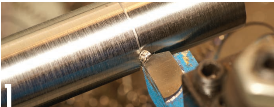
1 Turning involves reducing the diameter of a part by running a cutting tool along its length. The cutting tool is advanced into the work using the cross slide to take progressively deeper cuts until the required diameter is achieved. The tool is moved along the lathe bed using the automatic feed, the compound cross slide, or the carriage hand wheel.
