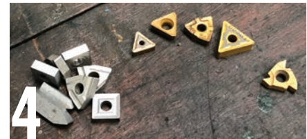
4 Indexable insert tools can be purchased individually, or in sets, which are often more cost-effective. The inserts are not sharpened when they are blunt, but are simply removed from the tool and rotated (or indexed) to use a fresh cutting edge. When all edges are blunt or damaged, the tip is discarded and a new one fitted. Tips are available in a wide range of types and typically cost around $10 each.
