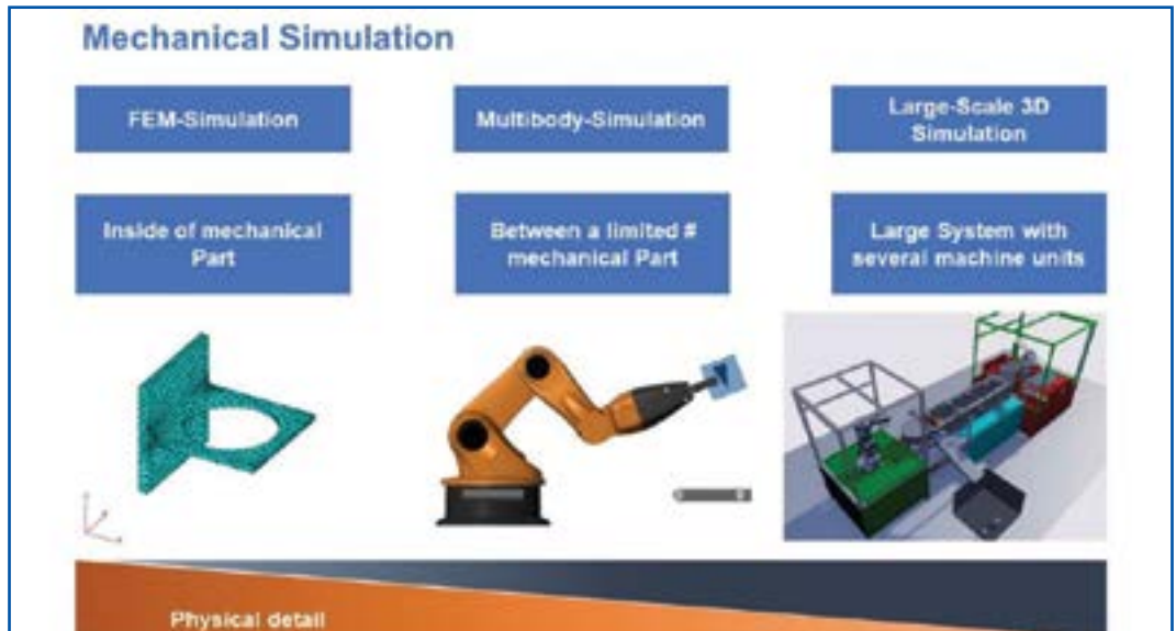
Figure 1: Existing ways of mechanical simulation such as FEM and multi-body simulations are usefully extended by 3D simulation with game engines. © 1984 - 2022 The MathWorks, Inc.
