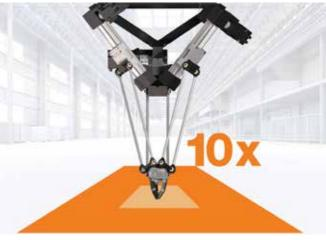
The delta robot from igus relies entirely on the advantages of motion plastics and enables simple, cost-effective automation. The new version has a 10 times higher working space diameter than the proven model.
