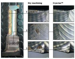
When viewed side by side, the improvement in the workpiece's surface quality is evident.
