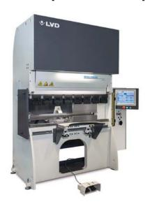
Fast setup with touch control: LVD's TOUCH-B 15-inch touch screen control makes setup fast and efficient. The CNC control minimizes operator input and makes part programming easy and intuitive. With minimal input, the operator can create 2D and simulate in 3D on the 15-inch touch screen. The LVD TOUCH-B control also offers network connection with LVD's CADMAN®-B programming software for added flexibility.
