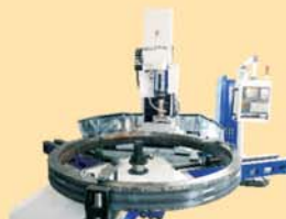
VIG-500 CNC VERTICAL INTERNAL GRINDING
