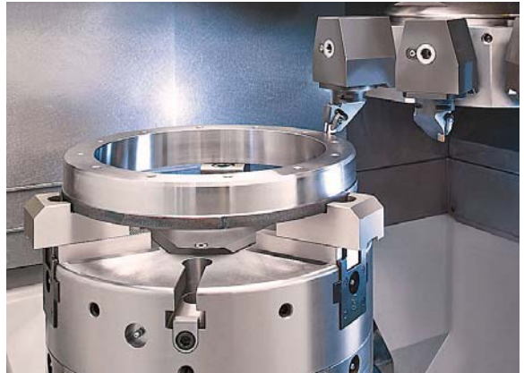
The bottom spindle can hold workpieces with a diameter of up to 450 mm. These are machined by the 12-station disk-type turret which can be fitted with both turning and driven tools.
