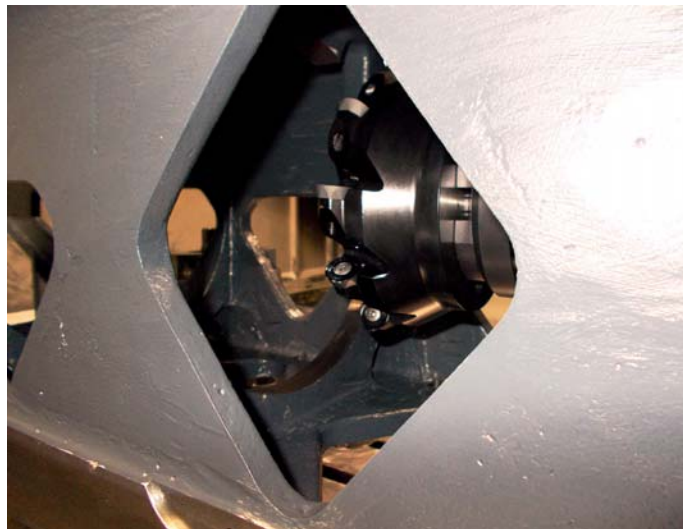
The F2334 round-insert milling cutter in front of the opening that is to be machined on the inside of the Z-slide. Image: Licon MT
