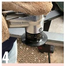
To use the tool, set the depth of the cutter and run it along the edge as shown. It works best if the travel direction is against the cutter direction, otherwise the cutter tends to dig in. Keep downward pressure against the part so the guide sits perfectly flat on the surface. While the tool produces no sparks, it does throw tiny sharp metal particles everywhere, so it pays to wear gloves in addition to standard protective gear.
