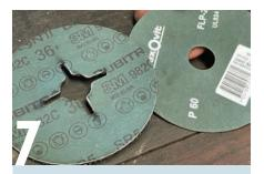
Choose a finer grit such as 60 for rounding edges and removing burrs. Coarser grit discs (such as 36 on the left) are more suited to bulk metal removal, smoothing welds and edge preparation for welding.
