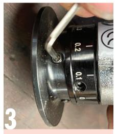
The rotating depth collar is locked into place with a grub screw. You need very little protrusion to do a good job – even 0.5mm is probably sufficient. You may need to check the graduations on the collar actually correspond with the protrusion of the cutter head (this can be adjusted if not).
