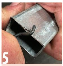
The tool is simply drawn along the edge in a scraping motion to cut the burr as shown.
