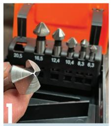
Holes require deburring or chamfering, even if it is only to help insert fasteners or ease installation of a tight-fitting part. This six-piece countersink set costs about \$74 and covers hole sizes from 1.5 to 20.5mm. It leaves a 45-degree chamfer on the edge of a hole.
