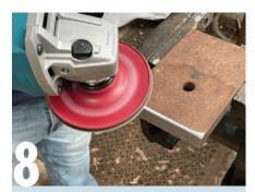
Use the fibre disc in the same way you would a flap disc. The backing pad should allow some deformation of the disc surface for smoothing and rounding over edges. Fibre discs are also ideal for rust removal.
