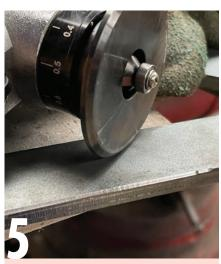
The pilot bearing controls the depth of cut, but will also reproduce any edge irregularities in the finished chamfer. The advantage of the pilot bearing is that once the depth of the bevel is reached, the tool will not cut any deeper if it is run back over the surface.
