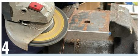
The beauty of flap discs over a standard grinding disc is they are flexible and can deform around the edge, helping create a rounded edge in the process. But they do wear quickly and at around \$8 a disc it can add up on big jobs.
