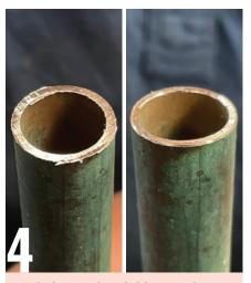
Simply place over the end of the pipe and rotate back and forth a couple of times. This Irwin brand tool costs about \$20.
