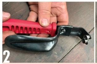
This sheet metal deburring tool costs less than \$20 and can quickly cut the burr off both sides of a sheet metal edge. Note the two cutting discs which need to be adjusted up together. They can be rotated and also reversed as they wear out.
