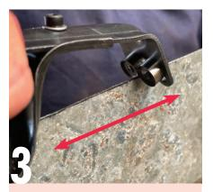
The tool is simply run along the edge of the sheet as shown. The guard over the handle will protect the hand from coming into contact with the rough edge.
