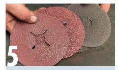
A potential cheaper option is to use fibre discs, as they are also flexible, and cheaper to purchase than flap discs. Single discs typically cost around \$3 but purchased in bulk the cost can drop to less than a dollar if you shop around. Grit sizes are similar to those available with flap discs and 125mm is the most common size.
