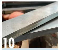
Laser cut parts can have very sharp edges, especially on thinner plate. Even the edge on this 6mm laser-cut plate is too sharp for general handling or painting.
