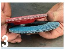
When purchasing flap discs, try to get a disc with an angled face (bottom) as opposed to a flat face (top). You will find the angled face disc requires less pressure to remove material quickly. This is more of an issue for bulk metal removal than simply rounding a few edges.
