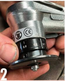
The small pilot bearing at the end of the spindle runs along the edge of the steel in the same way the pilot bearing on a router bit bears against the edge of a piece of timber. The rotary collar controls the depth of cut, or the protrusion of the cutter. The cutter itself is simply two indexable carbide lathe cutting tips (right). Note they can be rotated three times before they require replacement.
