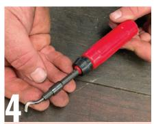
There are many styles of deburring tools with cutting blades, including small pen-sized tools that can be carried in a pocket, and telescopic deburring tools as pictured. The hardened steel hook-style cutting blades do wear out, but often the tools have spares stored in the handle.
