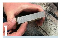
As mentioned previously, the choice of cutting method plays a big part in the surface finish and severity of the burr produced. Cold-cutting saws and metal bandsaws will produce the cleanest edge on thicker steel sections compared with abrasive disc drop-saws and angle grinders. The steel bar above only has a minor burr on the bottom edge from the bandsaw.
