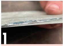
Sheet metal is one of the main offenders for producing razor-sharp burrs when cut. But the choice of cutting methods will play a large part in the severity of the burr. Pictured above are the results of cutting with an angle grinder and 1mm abrasive disc (top), and workshop sheet metal guillotine (bottom).
