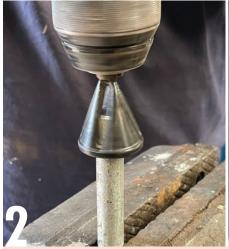
Simply touch it down over the end of a rod clamped in the vice and remove once the desired chamfer has been formed. These chamfering tools are also ideal for tidying up the end of threaded rod.
