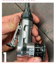
Possibly a better option is this air-powered chamfering tool, which costs around \$100 (we purchased ours online from ebay.com.au). For cleaning and chamfering the edges on laser-cut plate, the tool is absolutely ideal, and leaves a very neat 45-degree chamfer.
