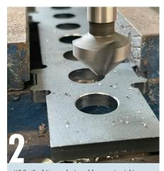
While the bits are designed for countersinking holes, they are also ideal for chamfering and deburring in the drill press, or even in a hand-held drill with care. Simply touch the bit carefully into the hole. It will tend to self-centre the part, so leave the part secure but moveable (for example, place in the drill vice but don't bolt the vice to the drilling table).
