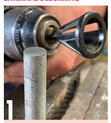
This eternal deburring tool is a little bit like a pencil sharpener for metal, and is placed in the chuck of a hand drill.
