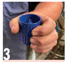
There are also deburring tools for pipe which work in much the same way and are hand-operated. The blue unit is designed for copper and PVC pipe so that fittings can slip easily over the end of cut pipe. It also includes internal deburring blades on the opposite side.
