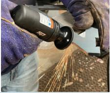
This small, compressed air-powered grinder is often used with 50mm surface cleaning discs for removing old gasket material from engine components. But 50mm sanding discs are also available, and are ideal for cleaning up edges on smaller components.
