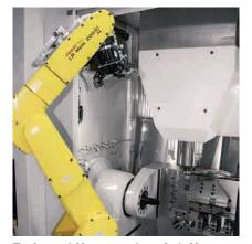
Thanks to variable programming and suitable devices, different parts can be automatically milled without set-up operation.
