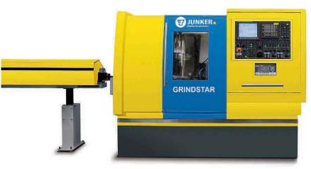
The Junker Grindstar is a dual-carriage grinding machine which combines plunge grinding with separation grinding.
