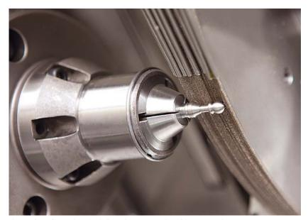
The use of a profile grinding wheel allows plunge-cut grinding of the entire workpiece contour, so minimizing the grinding time.
