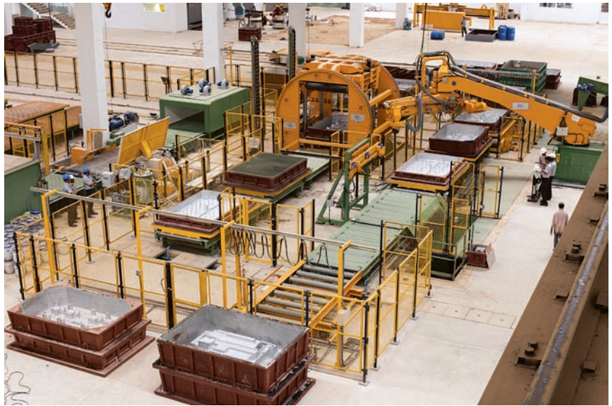
The foundry uses cake moulding so that the need for moulding boxes is eliminated
