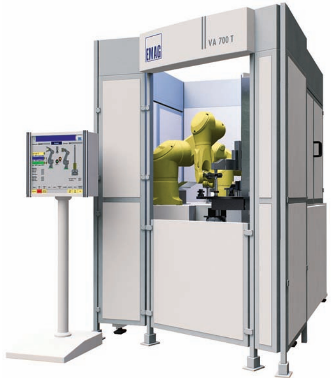
VA 700 T – Heat-shrinking assembly system for the manufacture of composite camshafts. Whilst one cam is heat-shrunk, the next one is already being preheated. Equipping the machine with a number of preheating units allows for optimal scaling of the application.
