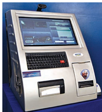
The E-gatepass system is an ATM type machine with a touchscreen, a camera and a printer.
