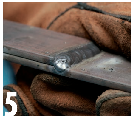
5 A lap fillet can sometimes be used in place of a simple butt joint, providing the design allows for the misalignment. The benefit of the lap fillet over the butt joint is it requires little preparation and can be welded on both exposed edges, giving greater strength.
