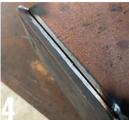
4 It is not always possible to form a corner fillet as shown previously. Here 75mm flat bar is being used to cap 75x125mm RHS, so it would be tedious to grind the edge of the bar down so a corner fillet could be welded. Better to form an outside corner V-groove, which leaves a neat joint with little clean-up required. If the sections were simply butted together, any welding would leave an overly rounded bead needing extensive grinding to clean up, also risking removing much of the weld in the process.
