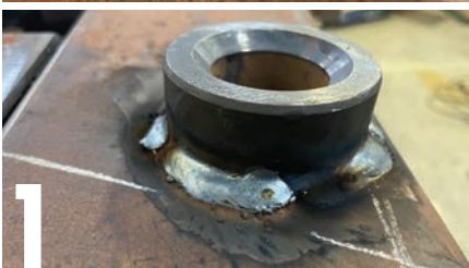
1 Fillet welds generally need little preparation (top), and any "veeing" of the joint can actually cause more difficulties when welding than simply cleaning the surface, although in certain situations it is required. Not all fillet welds are in a straight line! (Bottom).
