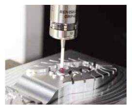
OMP40-2 machine tool probe
