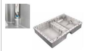
aluminium, ICN heads are designed with a sharp cutting edge and polished rake face. ICG heads feature a chip splitter for better chip removal when working with a long overhang. For drilling CFRP, special ICF geometry is available with diamond coating - this drilling head is designed to overcome all the typical CFRP machining failures such as delamination.
