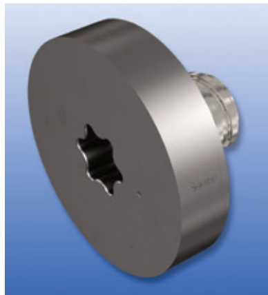
Fig. 4 – A disc-type blank head is ideal for customized solutions in milling slots and grooves. The hexalobular recess in a head face is intended for applying TORX-tipped wrenches with controlled torque for reliable clamping.
