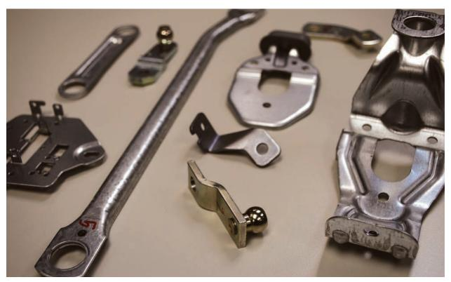
Eponsa produces all the stamped parts for windscreen wiper mechanisms
