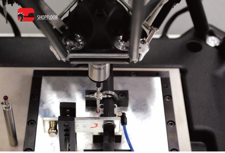
Equator has overcome difficulties of gauging a conical hole on a motor crank arm
