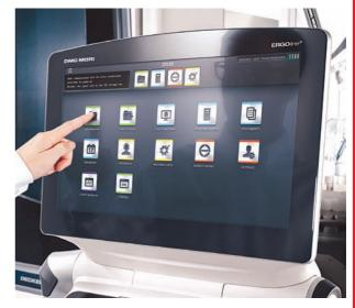
between the operator and the machine. Here, Celos displays up-to-date monitoring of the machine and and process. It supplies important key performance indicators for the current order as well as for the order progress. Moreover, it notifies the operator with special icons as well as text messages of any errors, problems or upcoming required maintenance work.
