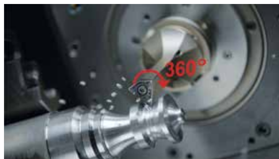
All contours can be machined in one setup, as the traditional turning operations of roughing, finishing, contour turning, face turning and longitudinal turning are all accomplished with a single tool.
