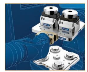
With the permissible pallet weights from 1 to 1,000 kg the Schunk VERO-S NSR robot couplings cover an enormous spectrum. For ensuring a process-reliable pallet change, every module is equipped with an automatic cleaning function now.
