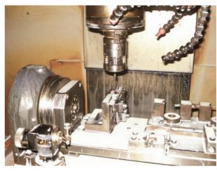
The OMP60 and OTS optical tool setting probe on a machine tool at Associated Tooling.
