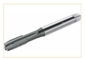
The Walter Prototyp Prototex® Eco Plus is the multi-talented tool among through-hole taps. A special pre-treatment gives the coating improved adhesion and therefore increases performance. The tool is also available as an option with internal cooling and radial coolant
