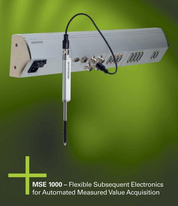
The HEIDENHAIN MSE 1000: Adapt the subsequent electronics modularly to the measuring task. You can use easily connectable modules for quick operability with digital or analog measured value data. Use freely configurable software—like Q-DAS—to display reliable quality parameters on the higher-level computer. This is how you can meet the high quality standard required in your industrial production.
