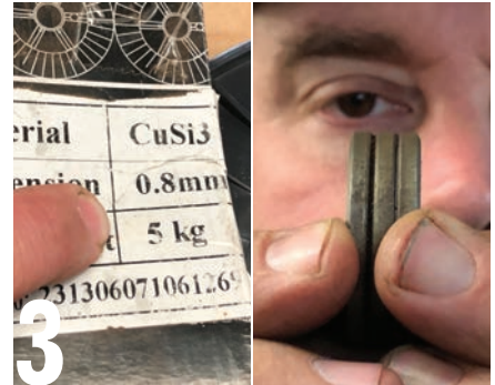
3 It is important to match the wire diameter with the drive roller groove. MIG welders are usually fitted with V-shaped drive rollers for regular mild steel welding, but U-shaped rollers as used with aluminium wire are best, as they are less likely to squash the softer wire.
