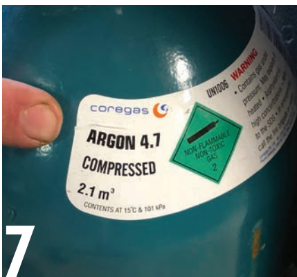
7 Make sure you are using 100 per cent argon, not 75:25 argon and CO 2 . Pure argon is commonly used with TIG welding and is also used when MIG welding aluminium.
