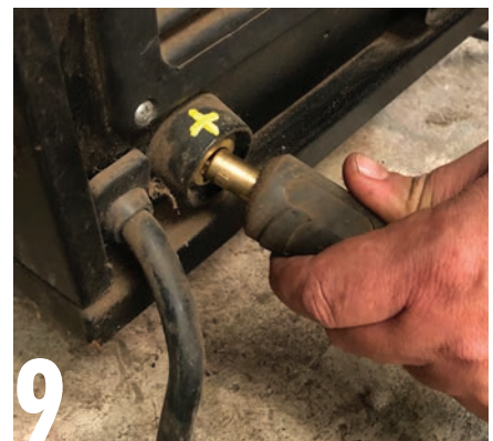
9 Finally, connect the welding electrode to the positive terminal, which is the same polarity as used with gas-shielded MIG welding. The earth lead should be attached to the negative post.
