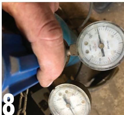
8 Adjust the regulator flow rate to about 12 litres per minute to start with. This can probably be wound back a little later to save gas, especially if there are no drafts in the workshop.
