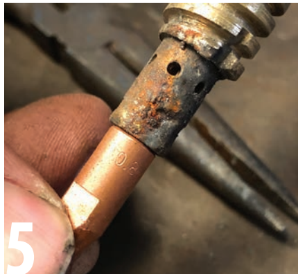
5 It is also a good idea to fit a new welding contact tip of the correct size when changing over to silicon bronze wire. But leave the tip off while feeding the new wire through to avoid it catching.
