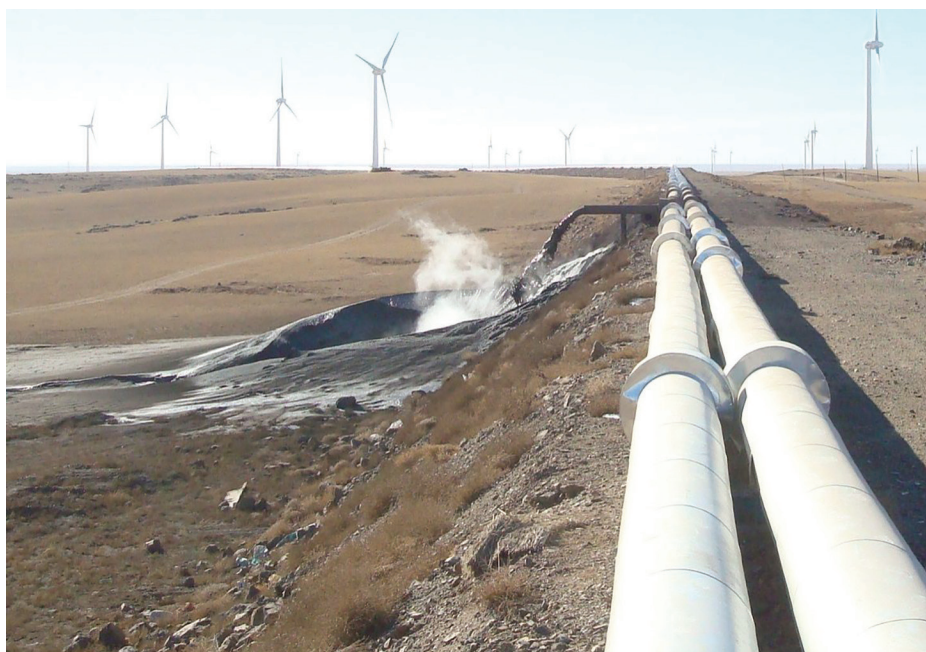
A thickened tailings disposal system
