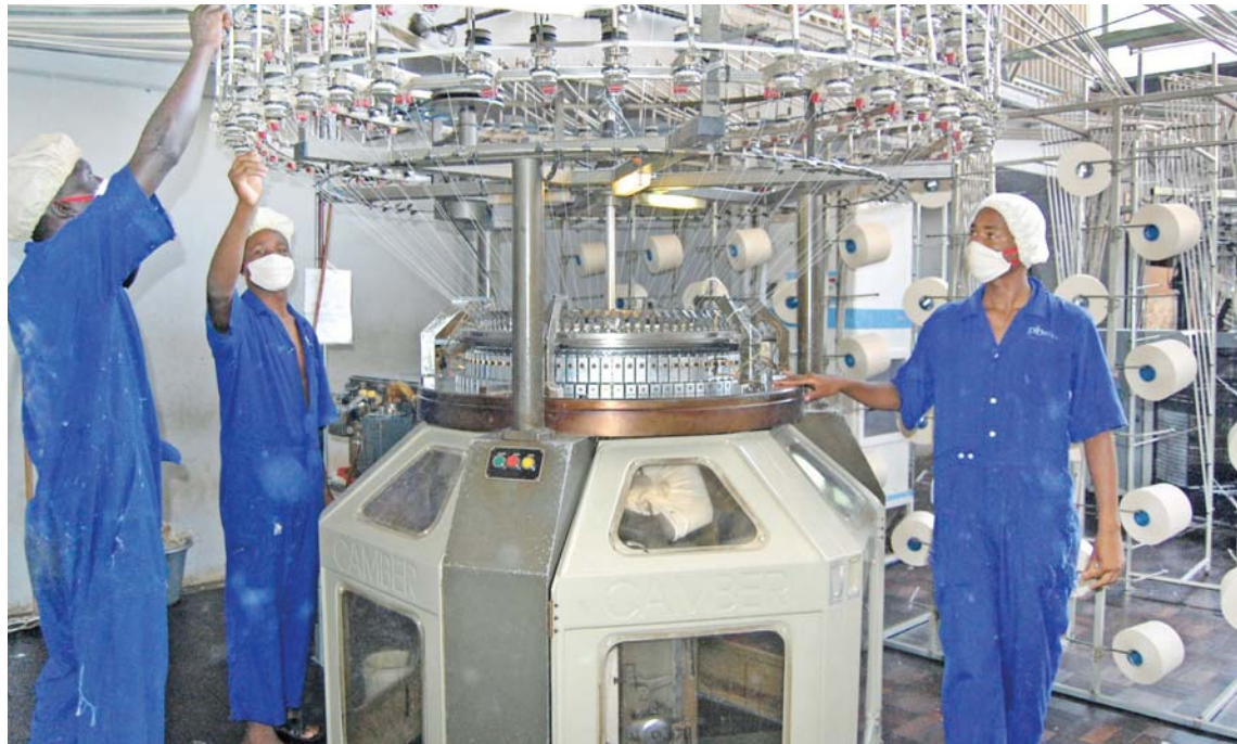
Workers in a factory operating machinery which stretches yarn used for fishnets
