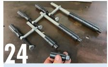
These threaded risers can be used to extend the clamp height for taller work and are simply screwed into the base of each clamp leg, before reattaching the 16mm adaptor.
