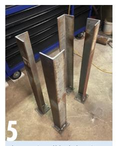
The next step is to weld the wheel mounting plates to the ends of the legs. While the positioning of the plates is not overly critical, make sure the holes have enough clearance for the bolt heads against the legs.
