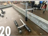
The key to the clamping system is the 16mm hole adaptors which simply screw to the base of the welding clamps (\$22 for a pack of four).
