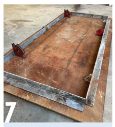
Even this 12mm plate needs bracing underneath to prevent flex. Our table frame has been cut from 65x65x6mm angle and squared up with the table edges. The legs will be attached directly to this frame. Make sure all frame members are straight and tack into position. Note the frame is set back from the edge, not flush with it which can impede clamping. It also keeps the wheels within the footprint of the tabletop.
