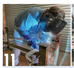
Here we are adding a second frame near the base of the legs to further stiffen the table. As an advantage, this frame can be used to mount a second shelf of mesh or thin plate underneath the table for storage. We have used some lightweight 50mm angle iron.
