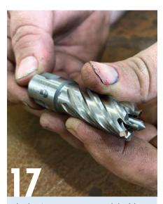
The clamping system uses a 16mm hole. If the tabletop is thick enough, the clamp is simply inserted into this hole without any additional securing method. As the clamp is tightened it grips in the hole, but it needs to be drilled accurately. For this job we are using a magnetic base drill with a 16mm rota broach (annular cutter). Note the centre locating pin which is used to line up the drill with the centre punch mark.
