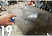
To finish off the table surface, we have cleaned it down with a wire cup brush in an angle grinder, then sprayed it with WD40, allowing it to soak in overnight. Any welding table in regular use probably won't have an issue with surface rust. The coating of penetrant will help stop welding spatter from sticking to the table surface.
