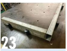
Even the insert stop pins are handy for laying out work when using the bench holes as a reference.
