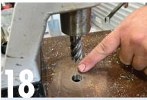
The rota broach leaves an accurate hole with a reamed-like finish. Depending on the number of holes you choose to drill, this may not be the quickest of jobs, so it may be easier to do a few every now and again until the job is complete. As our table is going to be used for strip downs as well as welding, only one end of the table will be drilled with holes.
