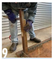
The legs can now be attached. Rather than try to clamp them at perfect right angles, we have simply attached them with a single large tack weld on the outside corner. They can then be adjusted for right angles by ben'ding or tapping with a block hammer and checking with a square as shown.
