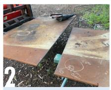
Any scrap metal yard can cut the tabletop to size for you, but they will invariably use an oxy acetylene torch. Here we have used the nine-inch angle grinder to trim the tabletop up. While this takes longer, the cut quality is far better and we have been able to spend some time making sure everything is square beforehand. Our table has ended up with a top about 1000 x 1800mm.
