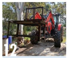
With the main body of the table now completed, it is time to turn it over and attach the castor wheels. Given the weight of the table, it is safer to carefully flip it with a tractor on soft sand to avoid damage rather than attempt to man-handle it.
