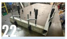
Clamps are simply inserted into the table holes and clamped down on the work. As our holes are accurately laid out, the base of the clamps provide a locating reference so our work can be easily set to 90 degrees. The same applies for 45-degree joins.
