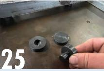
These magnetic rests are great for spacing work out when not all members can sit flat against the table surface. An alternative are these spacers which fit into the 16mm holes. In some cases, it may pay to raise the entire job off the table surface using these spacers, as it will allow welds to be run right down to the bottom edge without marking the table. Note that adjustable height spacers are also available.
