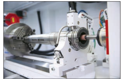
Internal grinding of tapers on long spindles.
