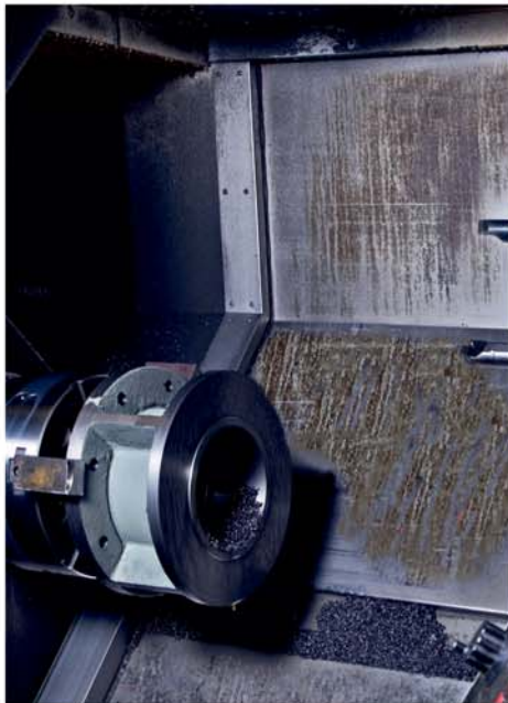
Scale formation with ordinary cutting fluid
