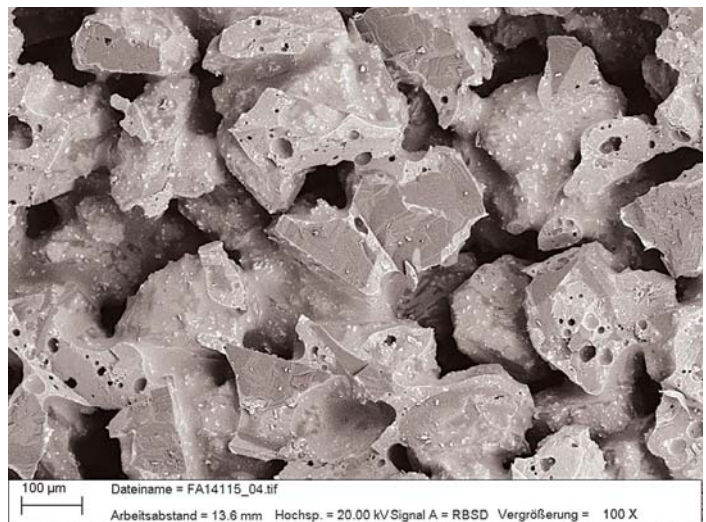
Optimum moistening of the GENIS 2 grain/bond matrix (source: TYROLIT)
