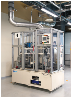
Stamping-type plating machine. Two machines installed on one bed. Each machine measures approx. 1x1x2 m (wxdxh).
