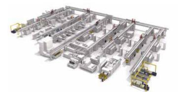
Pic 1 - Production plant for four-cylinder crankshafts in "herringbone" layout planned and supplied by BOEHRINGER as a turnkey project
