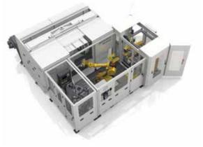
Pic 3 - Expansion of the shaft machining machines by a "MAG Cell" with automated workpiece measurement and material supply by pallets 10) Simulation and virtual commissioning of shaft machining with the software tools "NX CAM" and "Visual Components".
