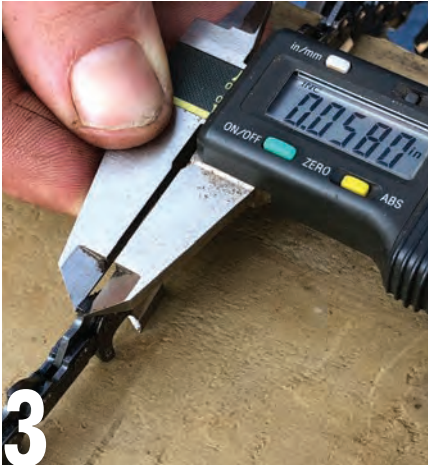
3 The tang on the bottom of the drive link rides in the groove in the bar and is a specific thickness or gauge; most often 0.050", 0.058" or 0.063", but sometimes you will find 0.043" on battery saws (eg Stihl Pico, Micro or Mini chain). The gauge of the chain must match the gauge of the bar. You can easily measure the gauge using vernier callipers as shown, set to imperial.
