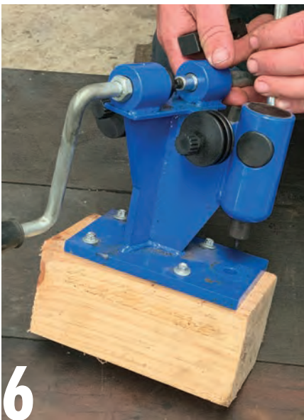
6 The main requirement for making your own chainsaw chains is a breaker and spinner tool. There are several styles available, and the unit pictured is one of the cheaper ones available (purchased online for around $120). While it is nothing fancy, the fabricated steel construction is certainly strong enough. As the name implies, it has dual functions of firstly breaking the chain, and then 'spinning' the preset rivets to join the chain. Rather than bolt it to the workshop bench, we have screwed it to a block of wood so it can be easily clamped in the vice.
