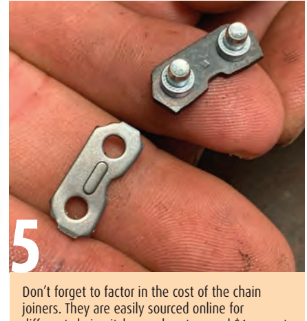
5 Don't forget to factor in the cost of the chain joiners. They are easily sourced online for different chain pitches and cost around $1 per set. They come in two parts: the tie strap (left) fits over the rear plate with the rivets (right) which is called a preset. You cannot recycle broken links that have been removed from a chain. While the tie strap could potentially be reused, it is often damaged from the breaking process. In the interests of safety only use new tie straps and presets when joining chain.
