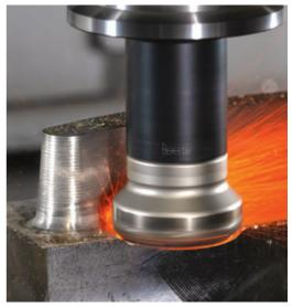
Fig. 3 – Milling cutters with indexable round inserts from ceramics provide considerably increased cutting speeds for higher productivity.
