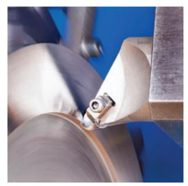
Fig. 1 – Superalloys are the key materials for turbojet and turboprop engines of modern aircrafts. Jet engine blisk machined with ISCAR's CUT-GRIP systems.
