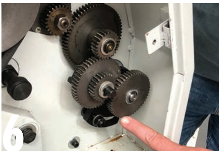
6 Lower cost lathes may feature a thread cutting gearbox with fewer options, while others may rely on a set of change gears to set the lead screw ratio of thread cutting. Most lathes will use some change gears in conjunction with the threading gearbox to expand the range of threads they are able to cut. When buying a lathe it is important to make sure it has the full set of change gears. It is also vital the thread cutting charts are included with the lathe, showing the change gear combinations to give the required thread pitches.
