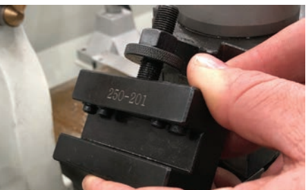
4 A quick-change toolpost (lathe) is great for increasing the speed at which work can be done on the lathe, as it allows tools to be swapped over in moments, and the tool height adjusted using a knurled nut, instead of using shims as with the standard turret-style tool post. It is important that a selection of tool holders (right) are included with the toolpost.
