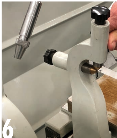
6 The travelling steady bolts to the carriage, and as a result travels with it. It is used to counteract the flex in a long, slender shaft when pressure from the tool is applied.
