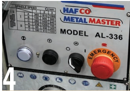
4 Other functions operated from the headstock may include (from left); Power indicator light, inching button (aids shifting spindle gear levers), coolant pump on/off, emergency stop button.
