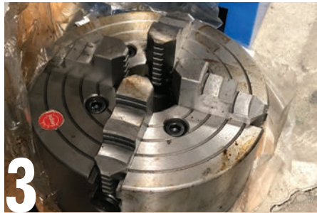
3 A four-jaw independent chuck is used to grip irregular-shaped work and should be included with any new machine. It is not self-centering, (although there are self-centering versions available), and jaws are individually adjusted. Note the chuck jaws are reversible to grip work from the inside or outside.
