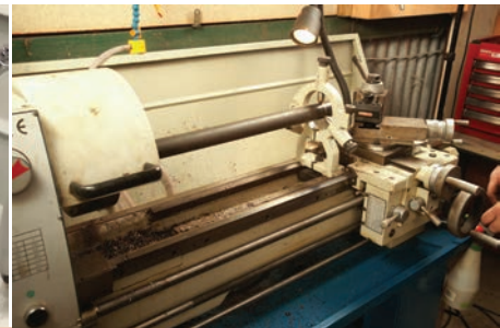
5 Steadies are attachments which are often missing from second-hand lathes, and difficult to replace if missing. There are two types - fixed and travelling. The fixed steady pictured is bolted to the lathe bed and adjusted up to centre and support overly long work. Like the headstock bore, it allows work on shafts which may be longer than the lathe bed. In the image on the right, the tailstock has been removed completely, allowing the shaft to be held in the steady and the end faced off.
