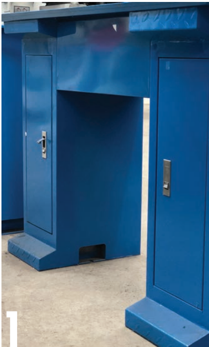
1 Unless you purchase a very small lathe, you will need a substantial metal base to hold the unit at working height. It is well worth purchasing a base at the same time as the lathe if buying new, as it will fit the unit in question and contain a sump for the use of a coolant system (if fitted). It's a good thing to check on the showroom floor as some units may include the base in the purchase price.
