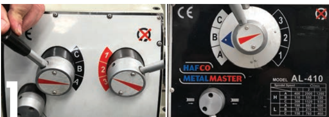
7 If we turn our attention to the headstock, examine the range of spindle speeds available. Small lathes or older units feature belt drive spindles, where speed is changed by switching the belt position in much the same way as a drill press. Larger lathes feature a gearbox with a wider range of spindle speeds from sub-100rpm to almost 2000rpm. The lathes pictured have nine speeds which are selected by two levers at the top of the headstock. Note the spindle speed chart; a total of 18 spindle speeds are available by changing the motor drive belt position.
