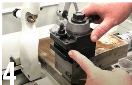
4 A quick-change toolpost (lathe) is great for increasing the speed at which work can be done on the lathe, as it allows tools to be swapped over in moments, and the tool height adjusted using a knurled nut, instead of using shims as with the standard turret-style tool post. It is important that a selection of tool holders (right) are included with the toolpost.
