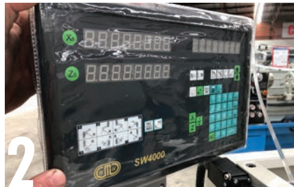
2 A digital readout is a handy addition and makes precision work much easier. It displays the tool position in X and Z coordinates, rather than relying on reading the compound and cross slide handwheels, which is especially good if your eyesight is strained by small numbers. Once again, it is probably cheaper to buy it fitted than attempt to fit one later on.
