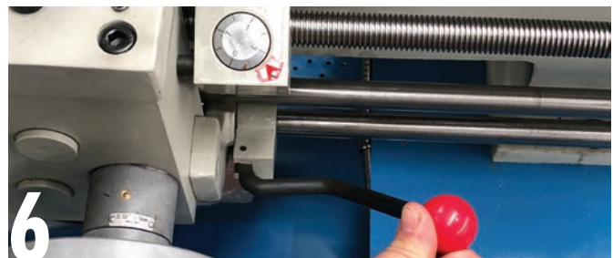
6 As mentioned previously, the spindle control shaft is operated by a lever which is attached to the lathe carriage. It is used to set the spindle in motion, as well as reverse its direction. Note the threading dial directly above the lever; it is engaged with the leadscrew and is used to reference the position of the tool when taking multiple passes when thread cutting.
