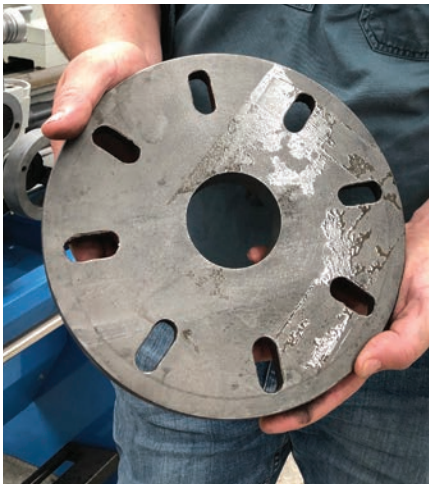
4 A faceplate should also be included with a new lathe. This is attached to the headstock in place of the chuck and is used to hold irregular-shaped objects, or where it is more convenient to bolt the object rather than grip it with a chuck.
