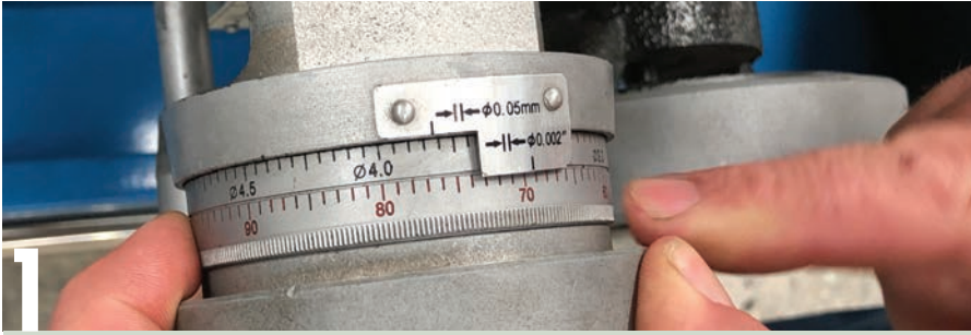
1 The metal lathe carriage houses a range of functions to manipulate the cutting tool (see Figure 2). The cross slide moves the toolpost in or out from the turning axis. Whether you work in the imperial or metric system, the cross slide hand wheel should feature graduations in both measurement systems. The same applies for the compound cross slide hand wheel.
