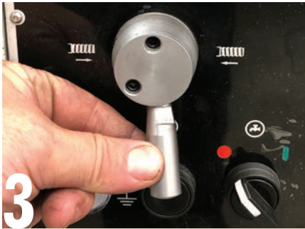
3 A range of other functions are controlled from the headstock. This lever is used to reverse the direction of the leadscrew for cutting left-hand threads.
