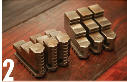
2 Three-jaw chucks should be supplied with a second set of external jaws which are fitted when gripping larger diameter work from the outside. Check they are supplied with any new machine.
