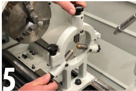
5 Steadies are attachments which are often missing from second-hand lathes, and difficult to replace if missing. There are two types - fixed and travelling. The fixed steady pictured is bolted to the lathe bed and adjusted up to centre and support overly long work. Like the headstock bore, it allows work on shafts which may be longer than the lathe bed. In the image on the right, the tailstock has been removed completely, allowing the shaft to be held in the steady and the end faced off.
