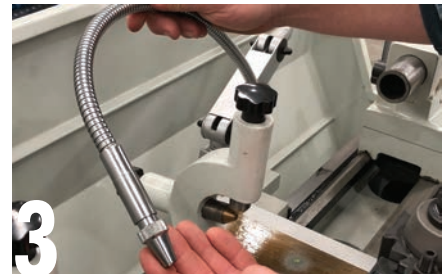
3 A coolant system is far easier to operate if it is integrated into the lathe and the base. While coolant is not absolutely necessary for lathe operations, it is a welcome feature if included in the package. This flexible nozzle is attached to the carriage and thus travels with the tool. A sump in the base plate collects used coolant and filters it into a reservoir before pumping it back to the nozzle.
