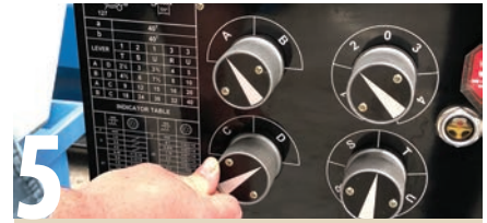
5 Apart from the spindle drive gearbox, the headstock houses the leadscrew drive gearbox, which is typically called the thread cutting gearbox. In some cases these gears will also alter the speed of the automatic feed. Gear positions are selected by these four knobs, giving a wide range of ratios and leadscrew speeds, which in turn give a range of thread pitches.
