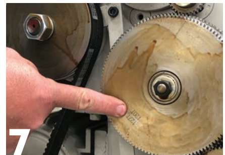
7 To cut certain metric threads on a lathe with an imperial leadscrew, and vice versa, a transposing gear featuring 120 and 127 teeth is used in the drivetrain.
