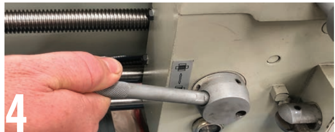
4 The split nut or half-nut lever engages the leadscrew for thread-cutting operations, which is the long threaded rod running the length of the bed (top left of picture). This locks the leadscrew to the carriage, moving it along the bed in the same fashion as the carriage auto feed. The leadscrew speed in relation to the headstock speed can be altered through a gearbox or series or change gears, giving a range of thread pitches for cutting different threads. Cheaper lathes use the half-nut as a form of carriage auto-feed.
